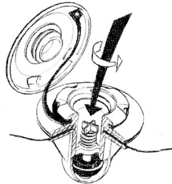
b) The valve is open.
