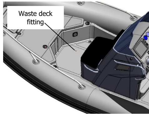
Fig. 51. Location of the waste deck fitting.
